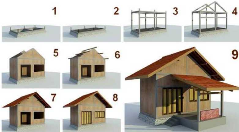
Figure 5. The Process of the Core House Construction
